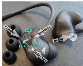
Figure 1: Image of the Hearpiece, including distances between microphones (centres of ports) and assigned microphone names.
